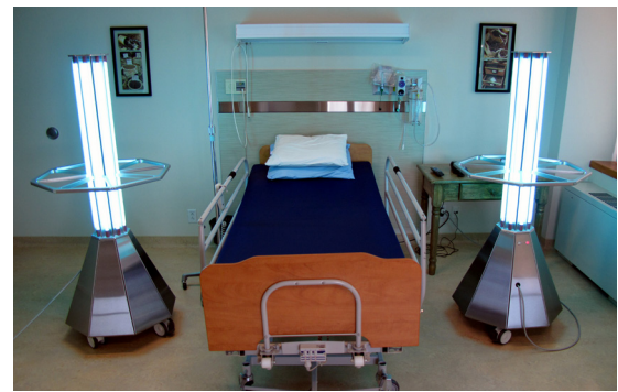
Example of a typical ASEPT.2X unit placement to minimize shadow areas
